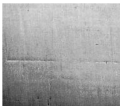
Scratch remains due to overload.
