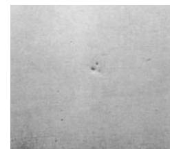
Pinhole texture by inappropriate rust proof.
